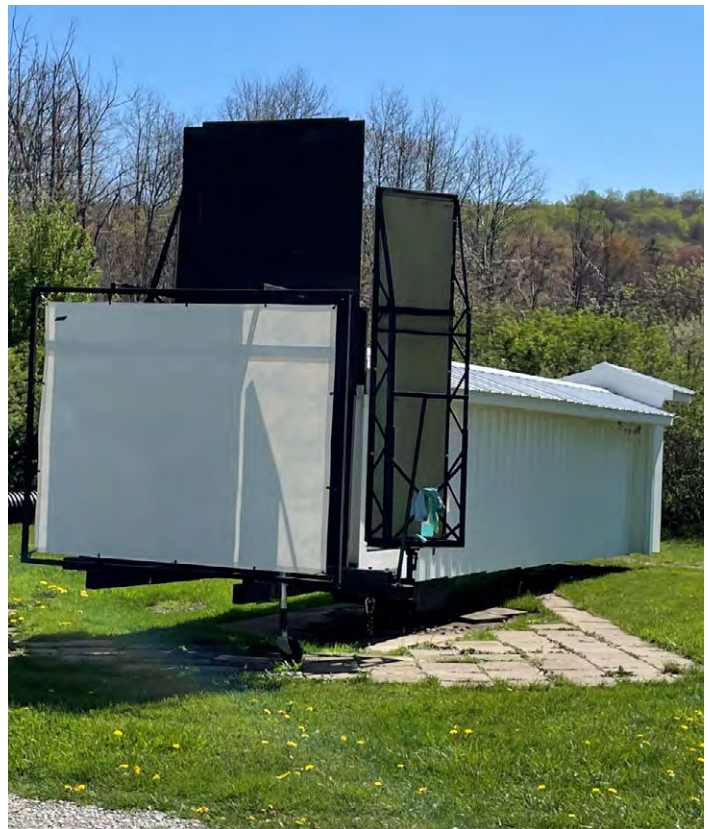
Specialized flight tunnel used for evaluating glazing products.
