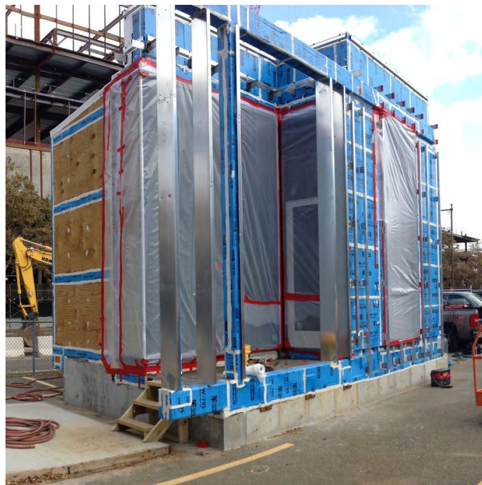
Full-scale performance mockup testing (75 | 125 Binney Street, Cambridge, MA).
