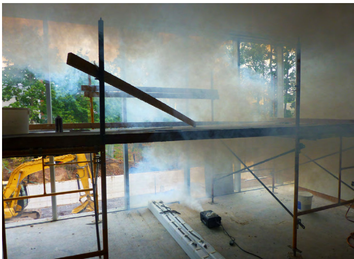
Air leakage testing with smoke (Hamilton College, Ruth and Elmer Wellin Museum of Art, Clinton, NY).
