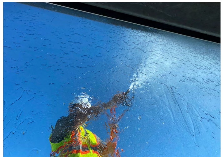
Water infiltration testing (Wellesley College, Wellesley, MA).
