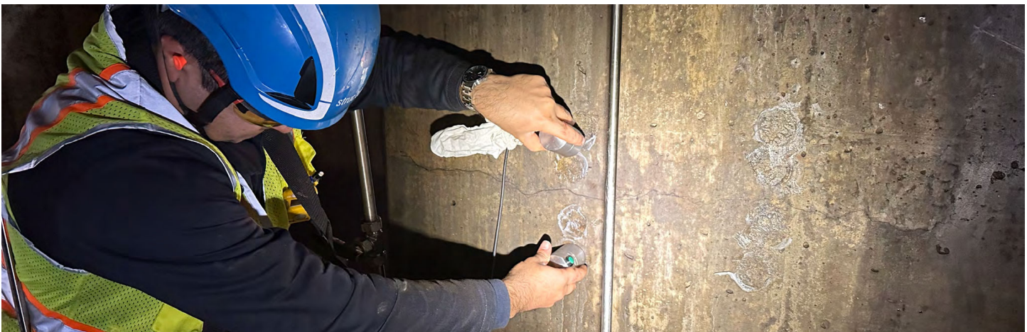
Performing UPV test on a machinery foundation to evaluate crack depths.
