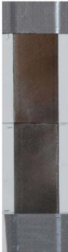
Cleaning with wirewheel
