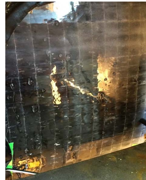
Specimen with multiple leaks at 150 psi
