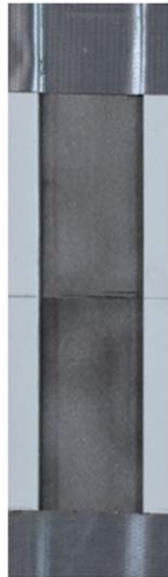
Sandblasting to SSPC SP-10 near-white finish
