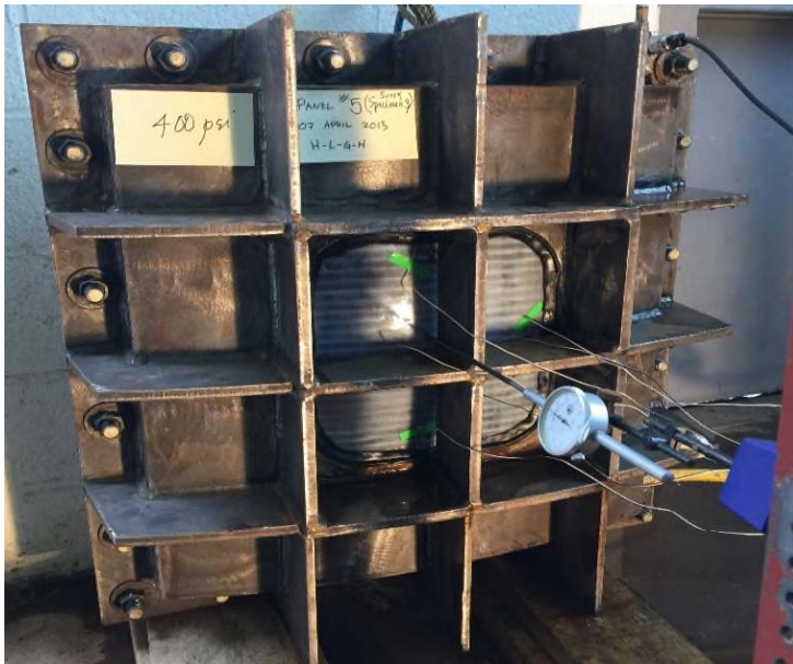
Specimen with no leaks at 400 psi
