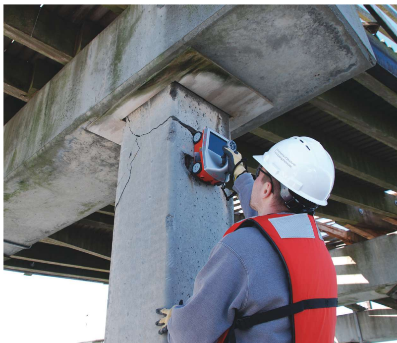
Fig. 8: Ground-penetrating radar (GPR) at affected piles
