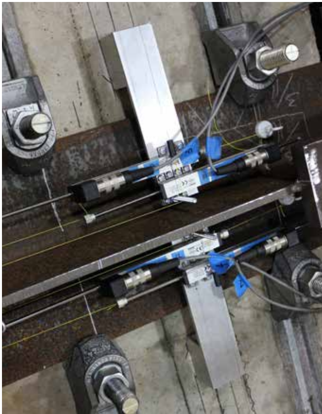
Figure 5. Push-out test specimen.
