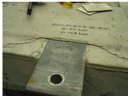
Figure 9 – Test BV24-24-6.4-1/2-7d-BCN with a bearing stress of 0.4f'_c .
