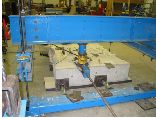
Figure 5 – Overall view of the test set-up showing both bearing and shear load application.
