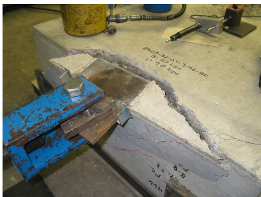
(a) Breakout showing the development of the rear crack behind the anchor plate. The studs are contained in the breakout concrete.
