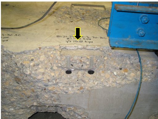
Figure 6 – Test BV21-24-6.4-1/2-7d-BC with a bearing stress of 0.1f'_c .
