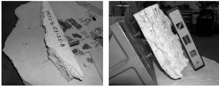
Figure 8: Concrete breakout failure for the two-stud anchorage
