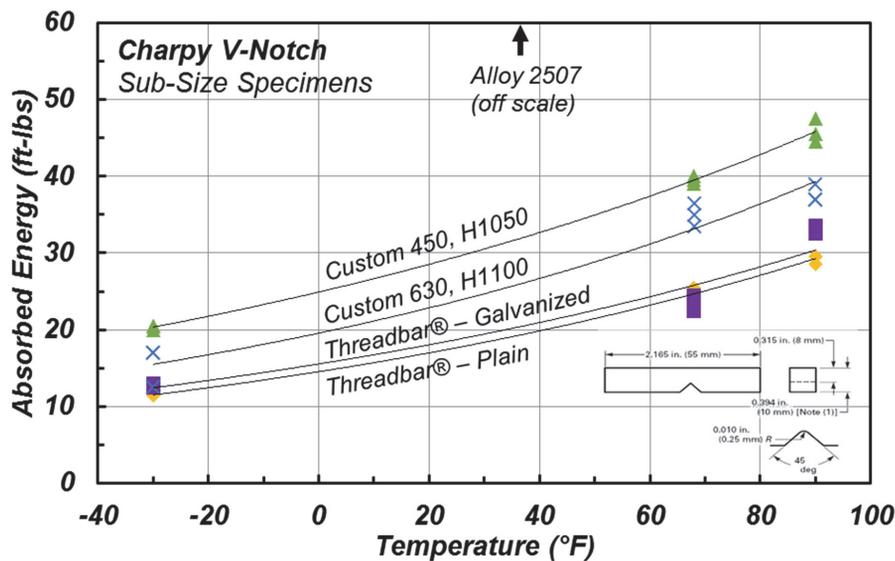
Fig. 6(d)—Charpy V-Notch, sub-size specimen test results (low range). (Note: 1 ft-lb = 1.355 J; °C = [°F - 32]/1.8.)
