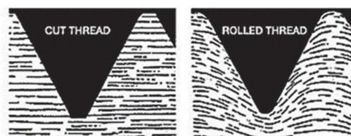
Fig. 2—Metallurgical differences in cut and rolled threads on bar as shown by modified grain structure (Reed Machinery 2014).
