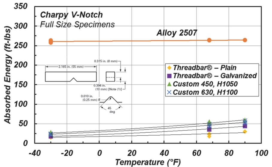
Fig. 6(a)—Charpy V-Notch, full-size specimen test results (entire range). (Note: 1 ft-lb = 1.355 J;  $^{\circ}\text{C} = [^{\circ}\text{F} - 32]/1.8$ .)
