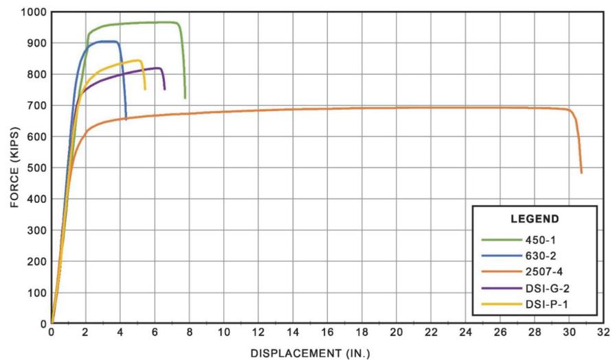
Fig. 4—Representative force-displacement curves. (Note: DSI-G-2 and DSI-P-1 bars had effective area of 5.16 in.<sup>2</sup>; other bars had effective area of 5.76 in.<sup>2</sup>; 1 kip = 4.448 kN; 1 in. = 25.4 mm.)
