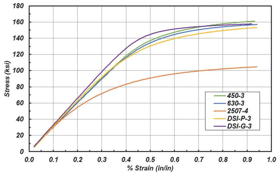
Fig. 3—Representative stress-strain curves prior to removing extensometer. (Note: 1 ksi = 6.89 MPa.)
