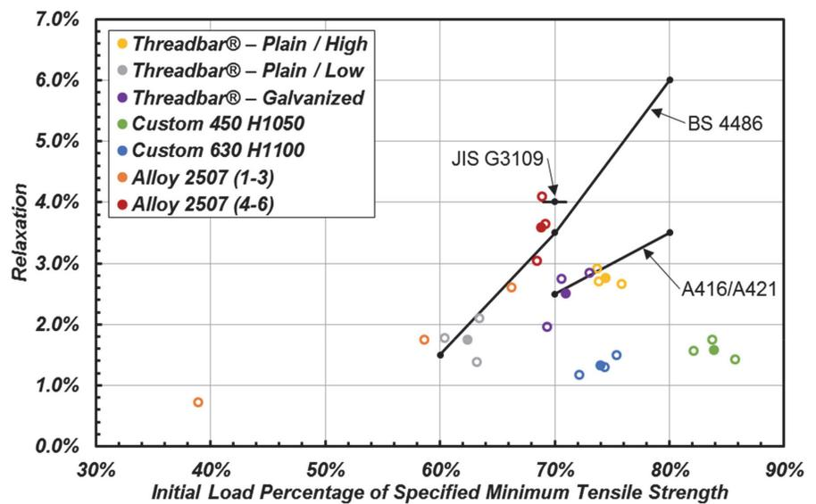
Fig. 5—Relaxation testing results compared standard limits (solid circles represent average relaxation from three samples; open circles represent individual test data).
