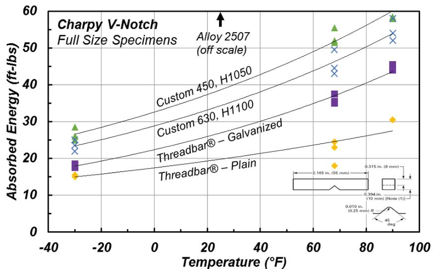
Fig. 6(b)—Charpy V-Notch, full-size specimen test results (low range). (Note: 1 ft-lb = 1.355 J;  $^{\circ}\text{C} = [^{\circ}\text{F} - 32]/1.8$ .)
