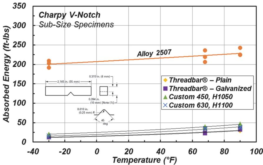
Fig. 6(c)—Charpy V-Notch, sub-size specimen test results (entire range). (Note: 1 ft-lb = 1.355 J; °C = [°F - 32]/1.8.)
