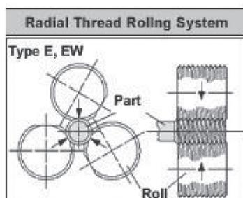
Fig. 1—Means of achieving threads on bar through cold-rolling (Koepfer 2003).
