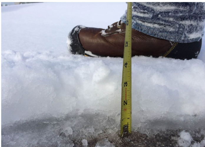
Varying densities throughout thickness of snow pack
