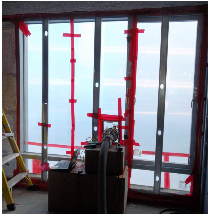
Air leakage testing
