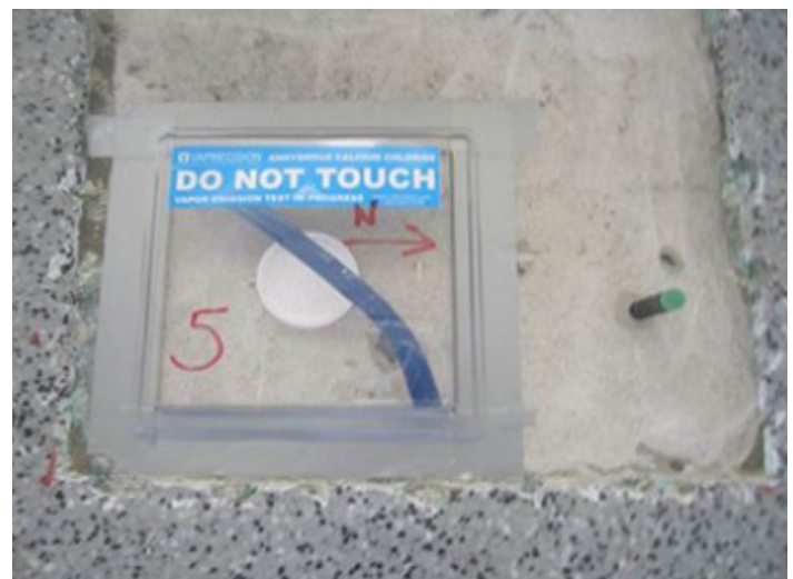
Moisture testing at floor slab with failed epoxy terrazzo finish
